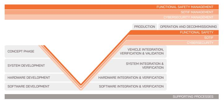
In addition to Functional Safety, the IDIADA team can deliver both Cybersecurity and SOTIF (Safety Of The Intended Functionality) services. This joined-up service is aimed at reducing the effort required to ensure the systems covered are both safe and secure.
