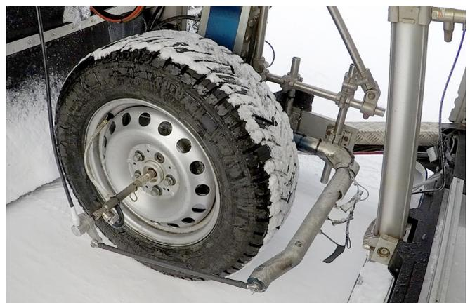
Apart from the characterization of tyre specific parameters, the skid trailer data can be used to measure proving ground adherence and to generate the tyre parametric models, such as FTire and MF-Tyre.
