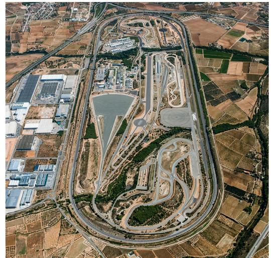
As part of these cutting-edge facilities, IDIADA has straight line braking surfaces, a test track part of the proving ground facilities. On this track, all kinds of braking from L-category vehicles are tested according to Regulation UN num. 78 and FMVSS122. In addition, there is an emissions testing laboratory which has been designed exclusively for L-category vehicles.
