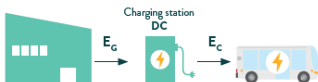
Charger efficiency test. (Picture from UITP 2014 standard)
